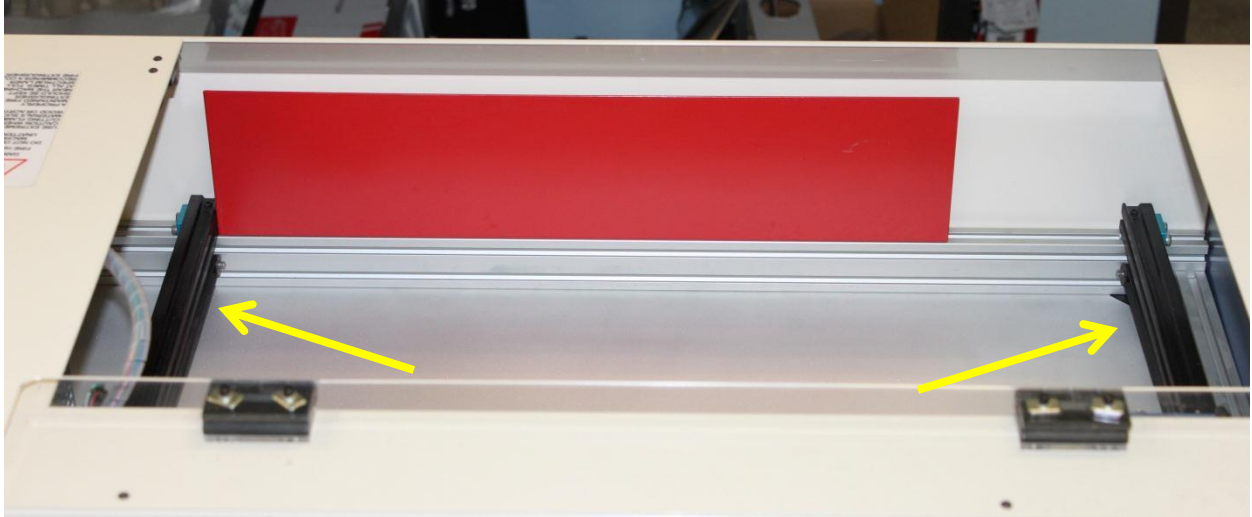
Figure 1 - Y rails (photo taken from back)
