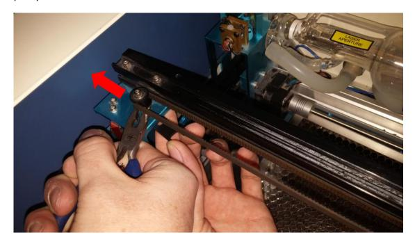
Once the idler pulley and hex nut are tightened, the belt installation is completed.
