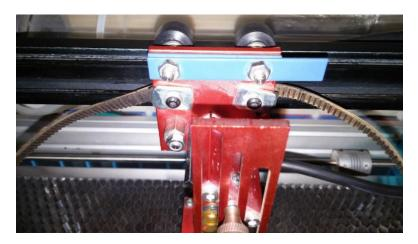
Once the belt is back into the laser head you can then put the belt back onto the motor gear on the right first and then place the belt onto the idler pulley on the left.
