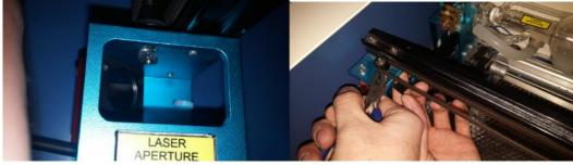
Once the hex nut is loosened the idler pulley will be able to be pushed to the right, loosening the tension on the x belt. You will then be able to remove the belt from the left side idler pulley.
