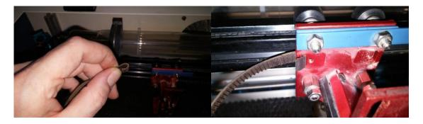
Repeat the process for the other end of the belt so that both sides are back into the laser head. You can then place the hex screw and t nut back onto each end of the belt securing them into place.
