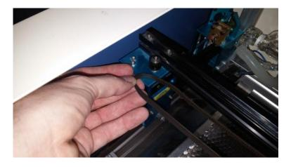
With the belt removed from the left side pulley you will not be able to remove the belt from the right side motor gear. This will allow the belt to be free from the idler pulley and motor gear and only be attached to the laser head. Now you can remove both the hex screws and t nuts holding the belt in place.
