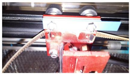
Once the hex screws and t nuts are removed you will be able to pull the belt out of its port in the laser head as illustrated below. To install the new belt, you will want to bend the end of the belt as illustrated below and enter it into the side of the laser head and the move the laser head to the right and left until the belt pops into the small port.
