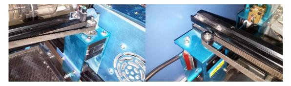
Once the belt is back onto the motor gear and idler pulley, you can now use the eccentric wrench to place onto the bottom hex nut under the idler pulley and then push the hex nut to the left. By pushing the hex nut to the left you are creating tension on the belt which you can then use the needle nose pliers to tighten the hex nut to the idler pulley and hold the tension on the belt.
