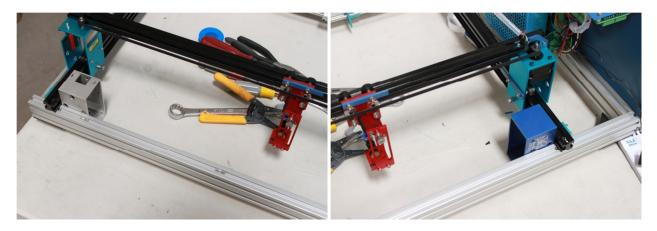
At this point loosen up the far right screw on the right coupler and the far left screw on the left coupler. Pull on the x-axis until both the left and right gantrys are level on the objects.
