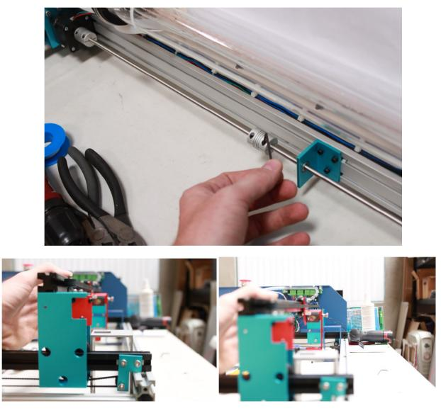
Once the x-axis is level simply re-tighten the left screw and right screw on the left and right couplers and the x-axis is in the correct alignment. Check by moving the x-axis up and down repeatedly and testing that both the left and right gantrys hit the objects at the same time. If they do not, repeat the process.
