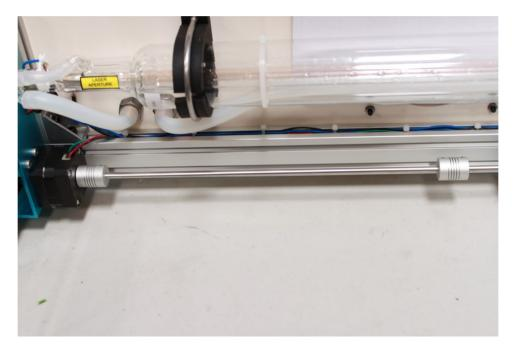
Then have two similar objects positioned against the insides of the black y rails. Then bring the x-axis down until one of the gantrys hit those objects.
