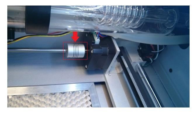
We'll want to loosen the two black allen screws on the above coupler. Next push the X gantry towards the rear of the machine. Keep pressure on the X gantry and retighten the coupler.
