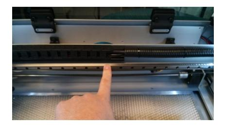
Once the coupler is tightened we'll want to bring the X gantry to the front of the machine and ensure the X gantry is square with the front left and right corners.
