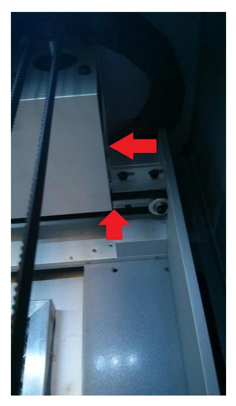
For the last step we'll want to move the X gantry after checking the front corners back to the rear to ensure it is square there as well.
