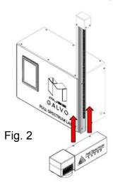
3. When rail is reached, manually align the rail opening and fasten them together until the scanhead is secure.
