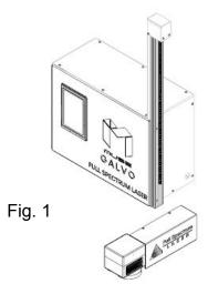
2. The scanhead (rectangular section) will be inserted bottom up.Make sure the wheels are lined up with the track.
