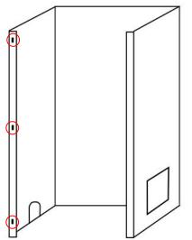
4. Connect the Bottom Support to front side of Enclosure using 4 screws, two on each side.
