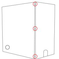
3. Attach the Left side to the back using three screws.
