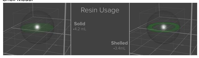
Shelling a model is a great option that will save resin and give your model inner structural support. The shelling feature will fill your model with a sturdy support structure while maintaining durable outer walls. This allows you to use less resin without compromising durability.
